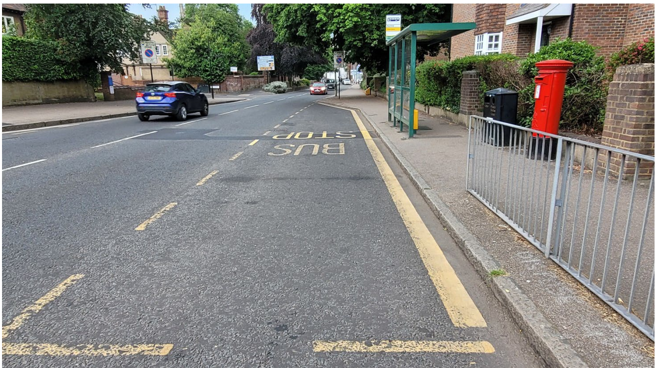
(Figure 10: example of bus bay / layby)
