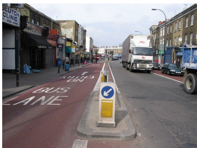
(Figure 15: contraflow bus lane)
