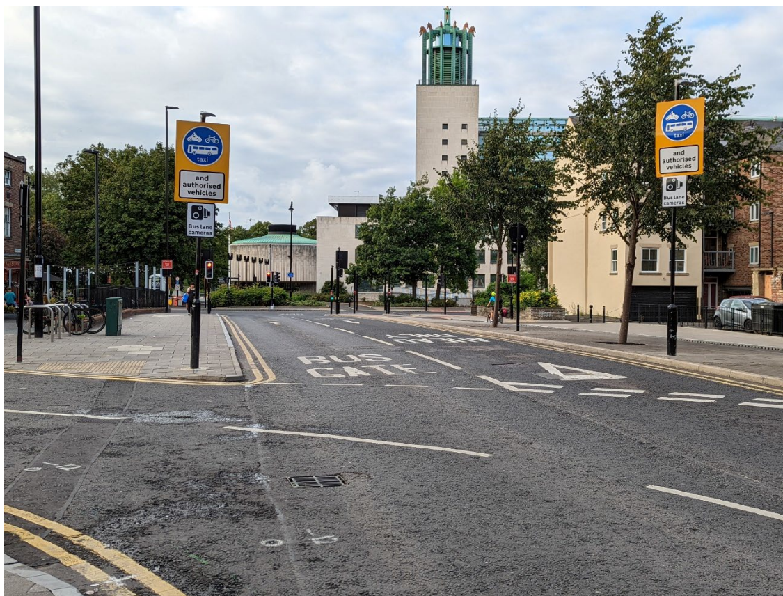
(Figure 24: bus gate with authorised vehicles permitted and camera enforcement)
